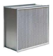
HEPA Filters are designed to meet requirements of very fine filtration up to 0.3 micron at high efficiency of 99.99 %. Due to hydrophobic & oleo phobic treatment on media, it does not allow any moisture & oil contents to pass through it.
